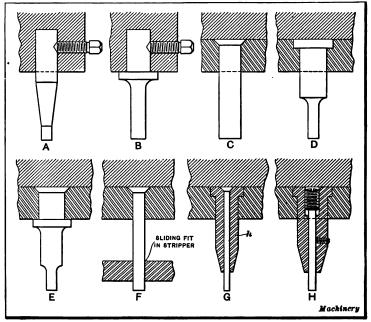
Fig. 22. Various Methods of Holding Piercing Punches
